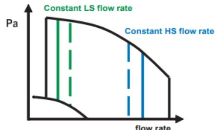
**DIVA** : proportional fan speed modulation on CO<sub>2</sub> levels.
