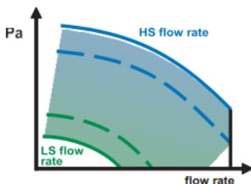
**QUATTRO** : proportional airflow modulation on CO<sub>2</sub> levels.
