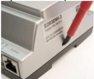
Press the clips on each sides of the box with a little screwdriver to open the the top of the box.
