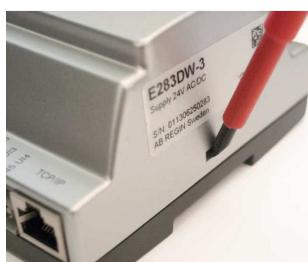
Press the clips on each sides of the box with a little screwdriver to open the top of the box.
