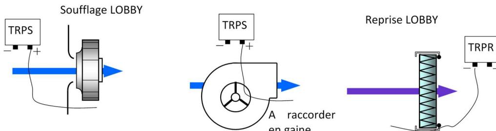
**IV.8. Pressure transmitter LOBBY® MAC2® QUATTRO® wiring and connection****IV.9. Motors wiring**
