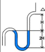
**Provide a siphon on each condensate drainage pipe.** A siphon can only be used for one drainage system. Note: the siphon must be connected in accordance with Best Practices in order that the condensates are removed as efficiently as possible.
