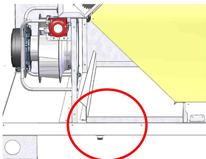
Manually lift the condensate pan to remove the screw in the coil. Then cut the wire feed on the underside to allow the coil to be positioned below the control panel as shown in the photo above. Be careful when cutting the wire feed that serves as a sealing washer.
