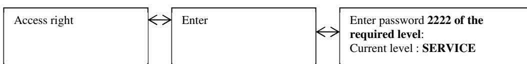
Enter **2222** with directional arrows and validate with OK. Press left arrow twice to reach the access of the menus. In case of mistake press C button twice and start again.
