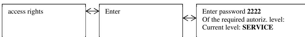
Enter the code **2222** with directional arrows then press the OK button. Press the left arrow twice to reach the menus. In case of mistake press C button twice and start again.
